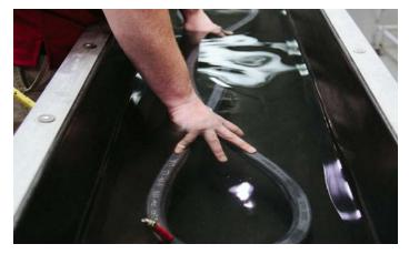
Each Seal Master product must pass a mandatory under water-leak test inspection, twice prior to shipment. Each part is inflated with a standard air pressure during these tests.
