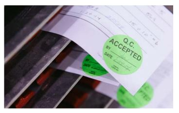
Each batch of material is assigned a unique identifier that allows for full tractability throughout production. By using the Seal Master serial number and the identifier of the material, finished products can be traced back to their original batch material.
