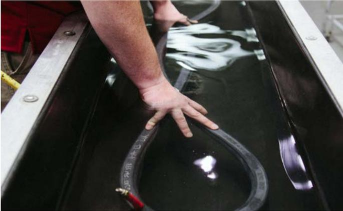
Each Seal Master product must pass a mandatory under water-leak test inspection, twice prior to shipment. Each part is inflated with a standard air pressure during these tests.
